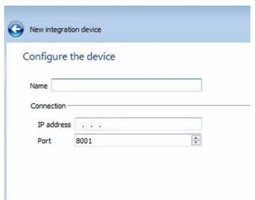
Enter Name, the IP address of the computer Herta is installed on, and the port number the information is being sent on. The default port number is 8001.
