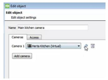
To configure overlays for each camera as needed, double-click the name of the camera and then click on the settings icon.
